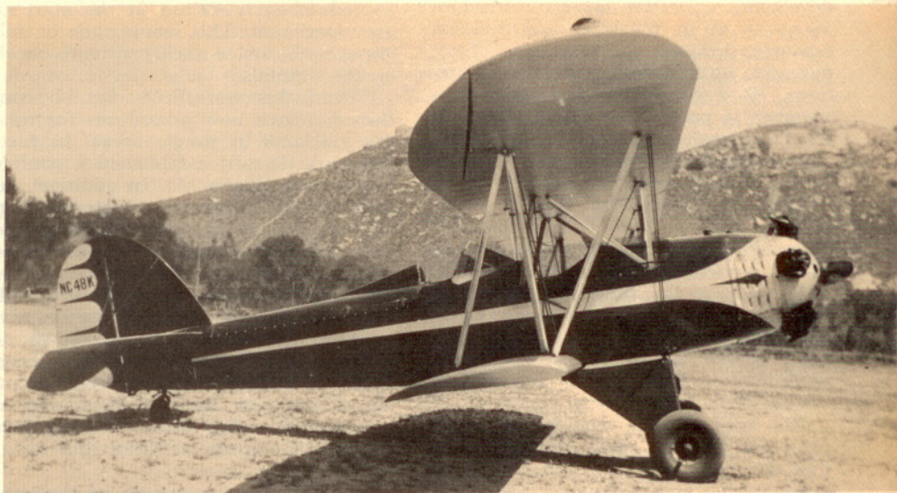
Bird C-K with 125 h.p. Kinner. When Birds were converted from tailskids to steerable tailwheels, the wheels were installed ahead of the original skid location. Filling in the landing gear struts as shown here was not standard practice.
