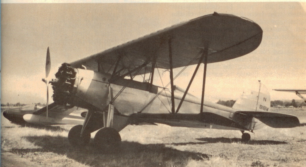
A Bird saved for better things. A C-K duster conversion, with single cockpit, 220 h.p. Continental W-670 engine, shortened lower wing with end plates, and modified landing gear, escaped the fate of most dusters and was used in the late 1950s for banner and glider towing. After towing the author's Schweizer 1-26A glider (background), the Bird's pilot assured him that he had to keep looking back to see that the glider was still on tow, since it had no noticeable effect on the towplane.
