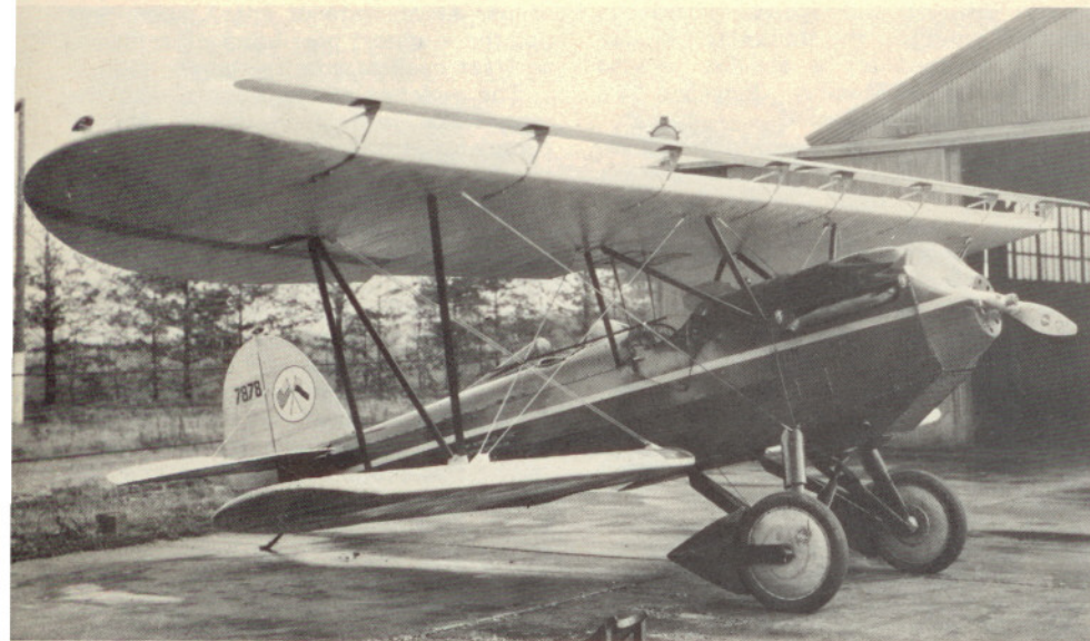
The modified Bird A entered in the Guggenheim Safe Airplane Competition. A full-span Ford-Leigh Safety Wing has been added to the upper wing, and thin wheels with partial fairings have been substituted for the fat airwheels that were standard equipment. Guggenheim photo
