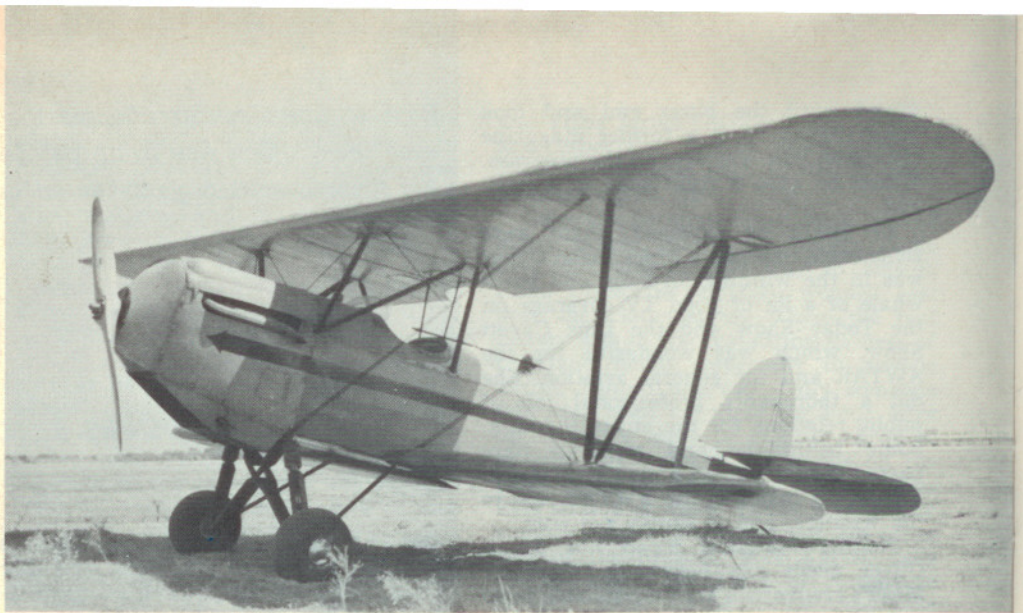
The Brunner & Winkle Bird Model A, with 90 h.p. Curtiss OX-5 engine. Note the radiator buried in the bottom of the nose in the manner of the contemporary Curtiss Hawk fighter. Photographed in 1941 still with its spring-leaf tailskid. Photo by Charles Schuler
